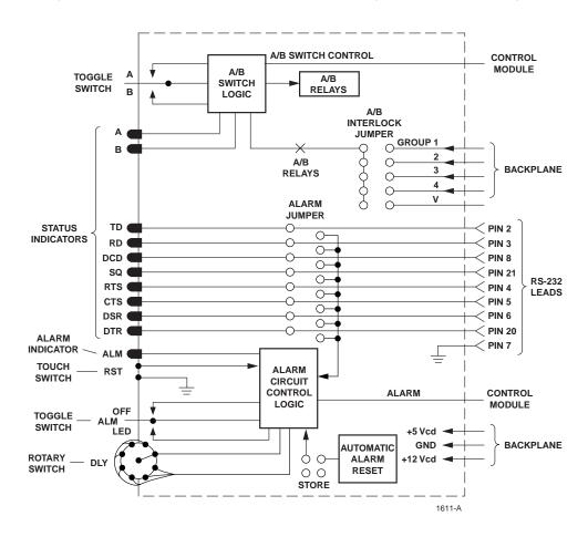
Figure 2-6. LED/Alarm Patch Module with A/B Switching Detailed Circuit Diagram
